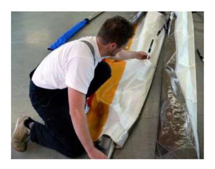
Push the rear sections of the leading edge tubes from the rear into the sail. Let the swivel tip exit the double sail at the zipper opening and push the tube into the front leading edge tube with the swivel tip cable pointing up. The swivel tip will swing to the rear. Press both snaps in and see that both snap out again through the holes in the front tube.
