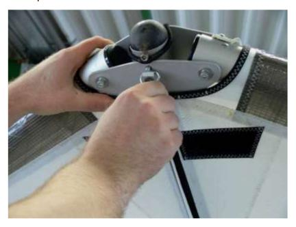
After this attach the snap hook of the spreader-bar safety cable from below = upwards into the tensioning line eye at the spreader bar; the zipper of the double sail is closed after this.
