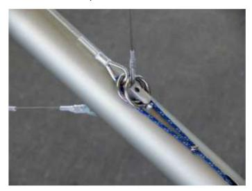
Then the steel ring of the rear upper rigging placed in the same notch. Check if the snap behind both rings is out and secures them.
