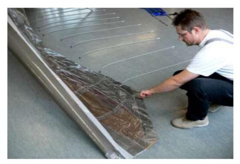
Red batten numbers = left side, green batten numbers = right side, looking in flight direction. [Portside and Starboard for the mariners] The batten quiver has separate pockets for the right and left wing. After the top battens are inserted, you can stand the glider up, if not done earlier, and tension it.
