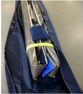
Lay down the short pack with the control bar area pointing up. Open the zipper and put the batten bundle [quiver] and both rear leading edge [wing tubes] to the side. If you are flying with non-split wheels, slide these on the speed bar now, before mounting it.
