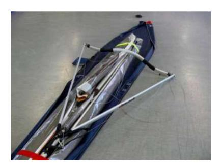
Now turn the wing over so it lies on the control bar and open the Velcro ties.
