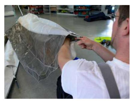
Then pull the wide, black, inside loop at the end of the sail leading edge over the endcap of the rear leading-edge tube. There is an auxiliary loop, which helps to do this. Pay attention to the proper seating of the loop webbing in the grove of the plastic endcap. Close the Velcro loop inside the sail to keep the black loop from moving out of its grove during transport.
