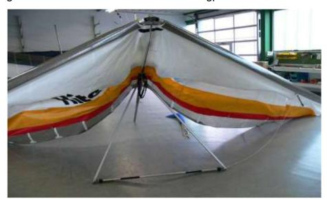
Spread the wings in steps, since the spreader bar has limited float.
