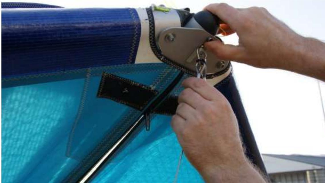
After this attach the snap hook of the spreader-bar safety cable from below = upwards into the tensioning line eye at the spreader bar; the zipper of the double sail is closed after this.
