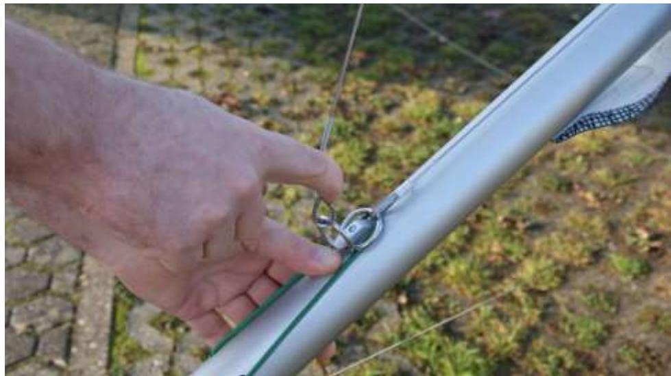
Then the steel ring of the rear upper rigging placed in the same notch. Check if the snap behind both rings is out and secures them.
