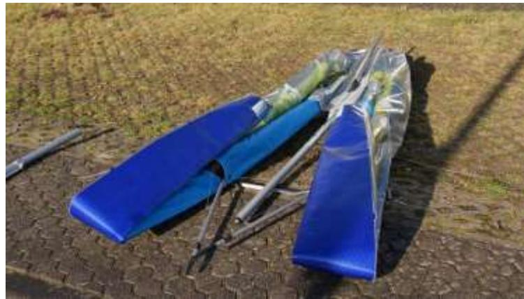
Lay down the short pack with the control bar area pointing up. Open the zipper and put the batten bundle [quiver] and both rear leading edge [wing tubes] to the side. If you are flying with non-split wheels, slide these on the speed bar now, before mounting it.
