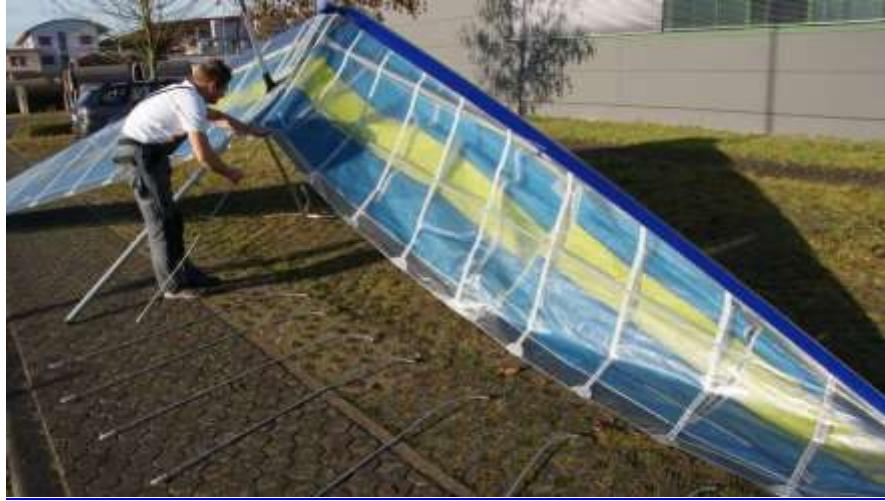
Red batten numbers = left side, green batten numbers = right side, looking in flight direction. [Portside and Starboard for the mariners] The batten quiver has separate pockets for the right and left wing. After the top battens are inserted, you can stand the glider up, if not done earlier, and tension it.
