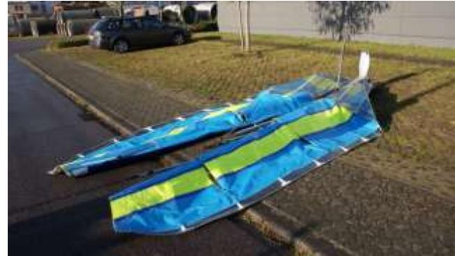
Push the rear sections of the leading edge tubes from the rear into the sail. Let the swivel tip exit the double sail at the zipper opening and push the tube into the front leading edge tube with the swivel tip cable pointing up. The swivel tip will swing to the rear. Press both snaps in and see that both snap out again through the holes in the front tube.
